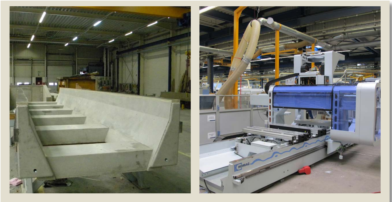
Figure 18: Production of machine beds for woodworking machines; left: UHPC machine bed; right: finished machine
