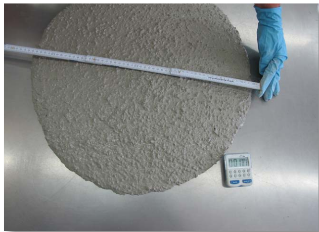
Figure 17: Slump of the UHPC mixed in the free-fall mixer
