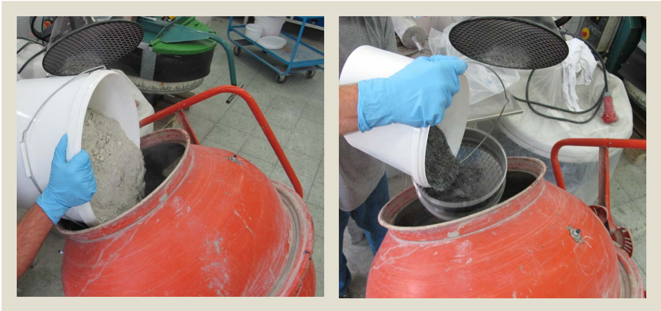
Figure 16: Addition of dry mix with NC 5941 (left) and micro steel fibres dosage (right)
